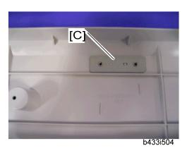
3. Attach the hand set support bracket [C] inside the scanner left cover.
