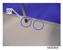
2. Make two holes [B] in the scanner left cover.
