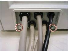
4. Reinstall the scanner left cover ( F x 2).
