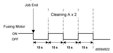
After the machine has completed printing a total of 6 to 49 sheets continuously (adjustable with SP3905-003: default 30), Cleaning A is done twice at the end of the job.
