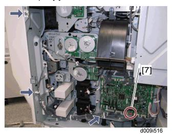
6. Connect the harness to CN211 [7] on the IOB ( $\stackrel{\frown}{\bowtie}$  x 3).
