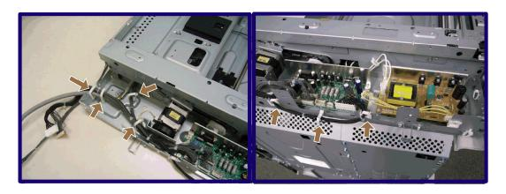
Scanner Accessibility Option B838 8. Remove the clamp [7] for the scanner I/F cable ( x 1). This clamp will be used hereafter.
